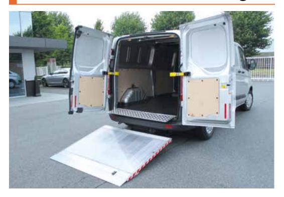
The DH-LSP was the first external lift ever in the tail lift industry, engineered to suit factory built panel vans. DHOLLANDIA still continues to lead the innovations in this field today. The intelligent shape of the lift arms eliminates the need to cut in the vehicle chassis or rear floor cross member, and maximises the ground clearance under the lift.
